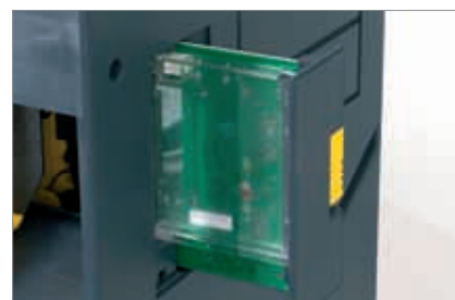
Optical sensor board easily extracted from the outside
